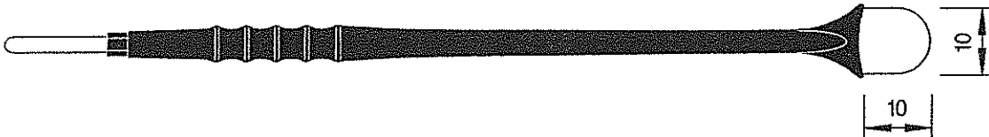
Wire Snare Electrode , 10 x 10 mm for the conization of the portio, circular, length 12 cm, single use, sterile. Package of 10 No. 20191-385
